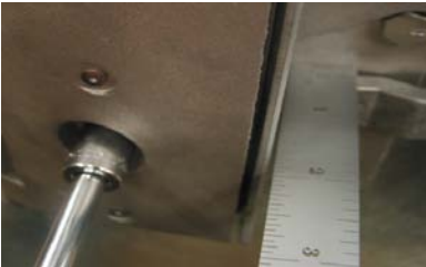
Fig. 9: Adjusting the LOWER SCREW (clutch retracting screw)
